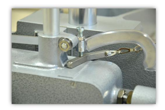
The sliding length (or 'footprint') is the distance that the rubber slider travels whilst in contact with the test surface. It is measured using the Perspex Setting Gauge.
