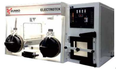
This range of workstations is ideal for the laboratory where oxygen free conditions are required for the growth and identification of bacteria. The careful configuration gives the units a small bench area yet ample working room within the incubator. The AW500TG is particularly economic to run due to its dual gas design, comes complete with catalyst sachets and plate holders and requires only electricity and gas supplies to be fully functional.
