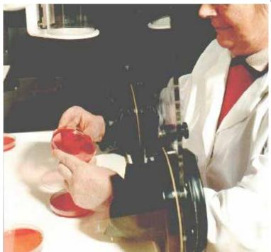
A large transfer port is fitted to the units which holds 60 Petri dishes. The outer door is hinged to reduce the overall length and the inner door slides to maximize the incubation capacity. Both doors are fitted with wear compensating seals. The units are also fitted with a single-plate entry system, situated between the arm ports at the front of the incubator. Individual Petri dishes can be passed quickly into the incubator with minimal gas usage.
