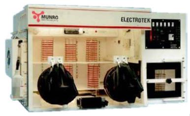
This range of workstations is ideal for the laboratory where oxygen free conditions are required for the growth and identification of bacteria. The careful configuration gives the units a small bench area yet ample working room within the incubator. The AW400TG is particularly economic to run due to its dual gas design, comes complete with catalyst sachets and plate holders and requires only electricity and gas supplies to be fully functional.
