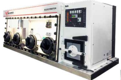
The AW800TGRF4P is the largest workstation in the Electrotek range. One of the main advantages of the unit is that despite its large capacity, it only occupies a modest amount of bench area. The workstation is very economical to run, as two gas supplies are used. The AW800TGRF4P will comfortably incubate up to 800 Petri dishes and comes complete with catalyst and plate holders.
