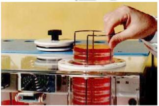
The positive pressure inside the incubator and the doors at each end of the locks together with fast acting gas inlet switching, ensures that the unit remains anaerobic at all times.
