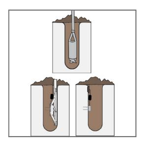
**2. Check Sensor Operation -** Plug the sensor into the data logger and use the SCAN function in the software to do a quick check of sensor operation before backfilling.
