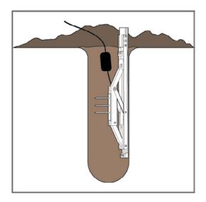
**2. Check Sensor Operation** - lug the sensor into the data logger and use the SCAN function in the software to do a quick check of sensor operation before backfilling.
