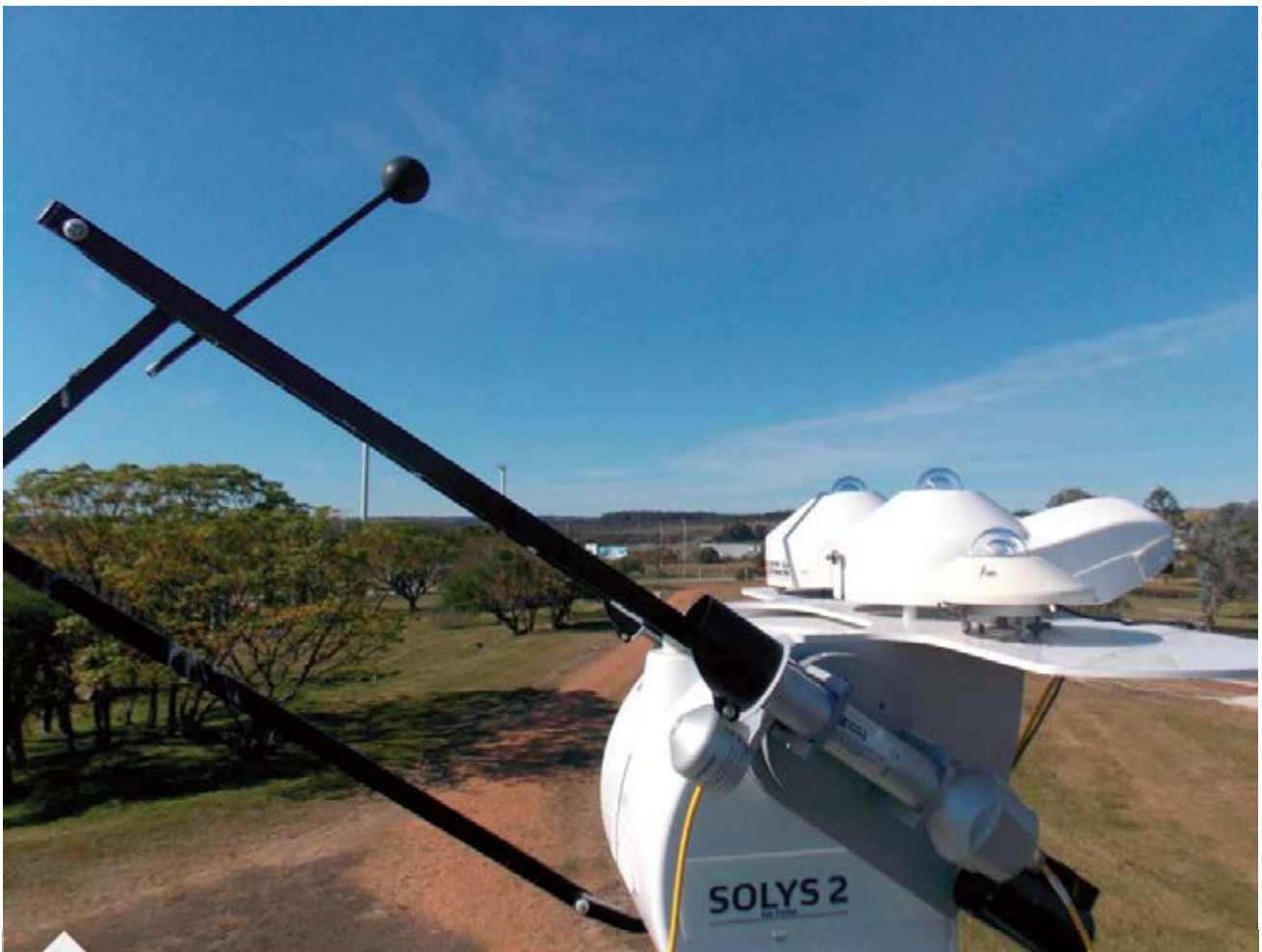
Continuous irradiance measurements with radiometers mounted on a SOLYS2 sun tracker at LES
