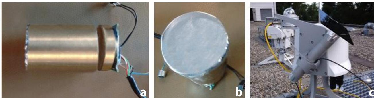
**Figure 2** (a) Pointing accuracy apparatus consisting of a brass tube with a pinhole in aluminium at the left and a CMOS camera at the right end, (b) aluminium foil with pinhole, and (c) the pointing accuracy apparatus on the RaZON<sup>+</sup>.
