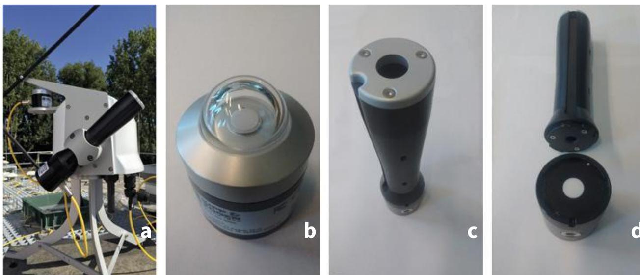
**Figure 1** (a) The RaZON<sup>+</sup> at the measurement location, (b) the RaZON<sup>+</sup> PR1 pyranometer, (c) PH1 pyrhelimeter, and (d) PH1 collimation tube separate from detector unit.
